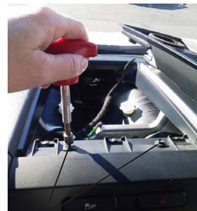
Screws to remove radio bezel
