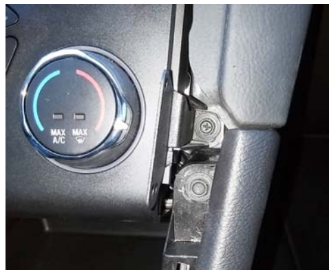
InDash installed showing screw location
