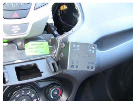
Mount installed showing screw location
