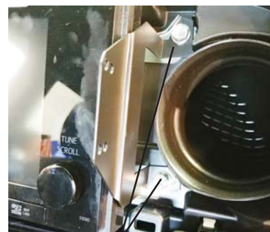
InDash showing (2) mounting bolts placement.
